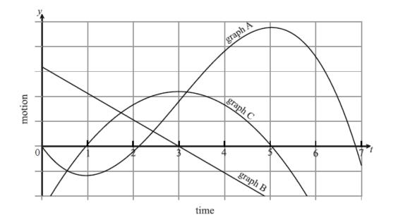
The following diagram shows the graphs of the displacement, velocity and acceleration of a moving object as functions of time, t.
